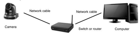
2. To connect directly through network cable, the IP address of the computer should be changed so that it is on the same network segment as the camera E.g.: The factory-preset default IP address of the camera is 192.168.100.100. The computer IP address must be set with the same network segment, such as 192.168.100.101, so that the computer can be connected correctly with the camera
